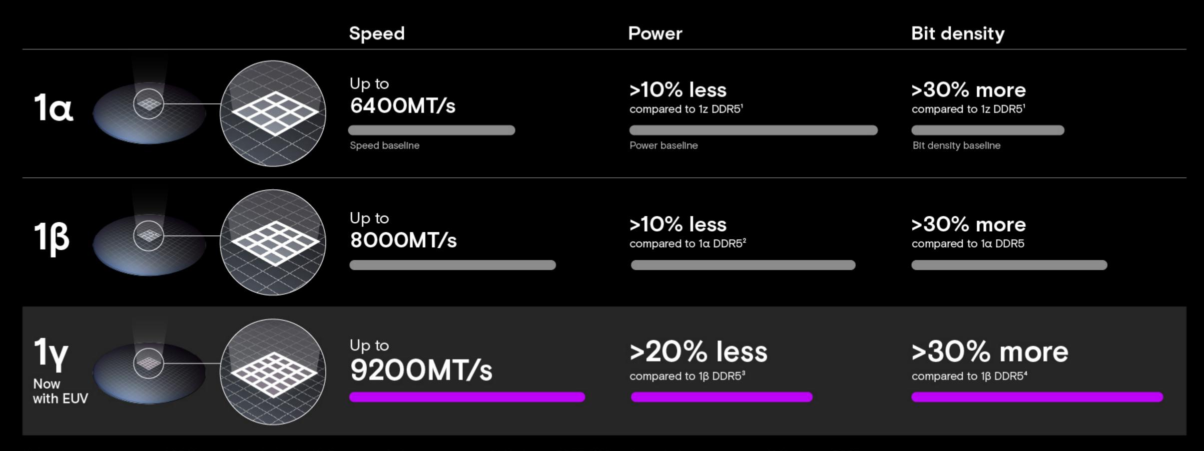
(1) 1z is the previous version of DRAM technology before 1α. (2) Based on calculations comparing 24Gb density DDR5. (3) Based on calculations comparing 16Gb density DDR5. (4) Calculated based on overall bits per wafer comparing 1β and 1γ process.
